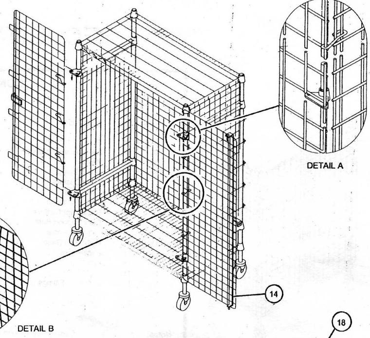
**13.** A) Check Door and latch pin operation by first closing the left door (A), then the right door (B), and sliding the latch Bar down (C). The Top and bottom Latch Pins should pass between the wires on the top and bottom shelves, preventing the Doors from opening. (See details.)
