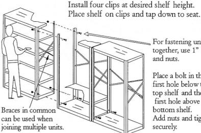
For fastening units together, use 1" bolts and nuts.
