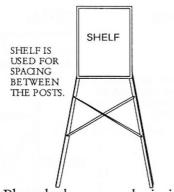
Place the braces on the inside of the post. Insert 1/4 x 1/2 long bolts from the outside of the posts. Attach nuts and tighten.
